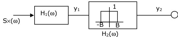
PSD of input  $S \times (\omega) = N_o$  W/H2.  $H_1(\omega) = 2e^{-j\omega t d}$
