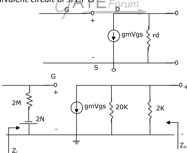
$$Z_i = 2M; Z_{out} = 20k \parallel 8k = \left(\frac{20}{11}\right)k\Omega$$
