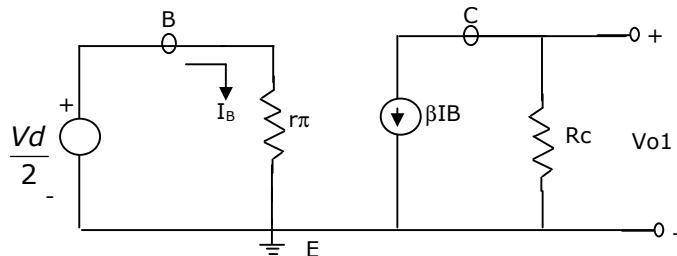
$$A_d = \frac{V_{o1}}{V_d} = \frac{-\beta R_c}{2r_\pi} = -\frac{g_m R_c}{2}$$
